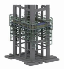
水泥预热器塔架结构爬升施工装备 Climbing construction equipment of cement preheater tower structure
